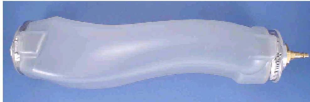
Figure 3: The mandrel is cooled below the transition temperature resulting in a rigid mandrel.
