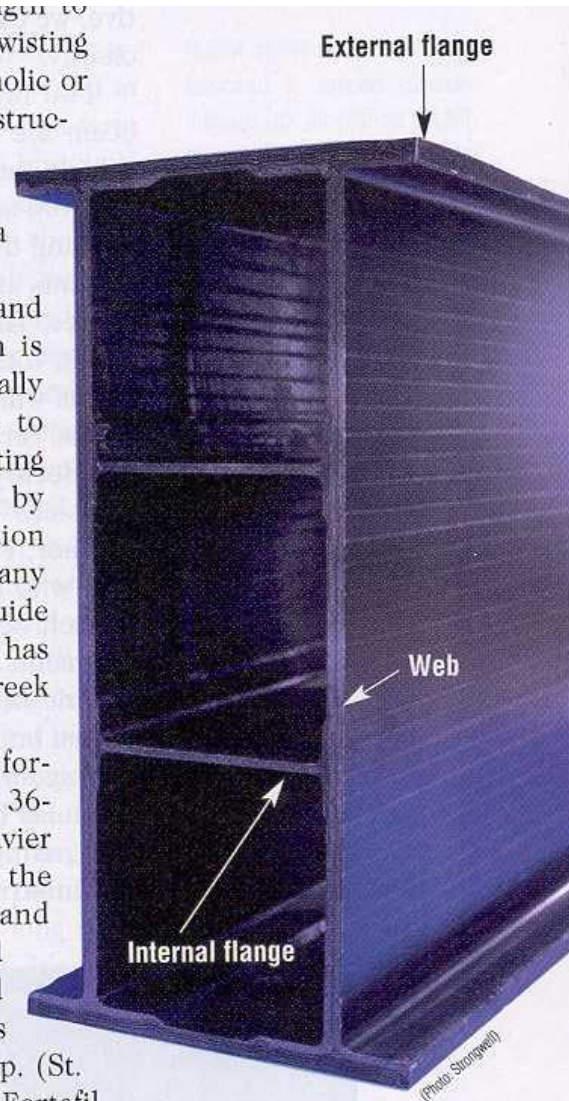
Strongwell's pultruded double-webbed internally-flanged 36-inch composite beam incorporates carbon fiber in the top and bottom flanges.
